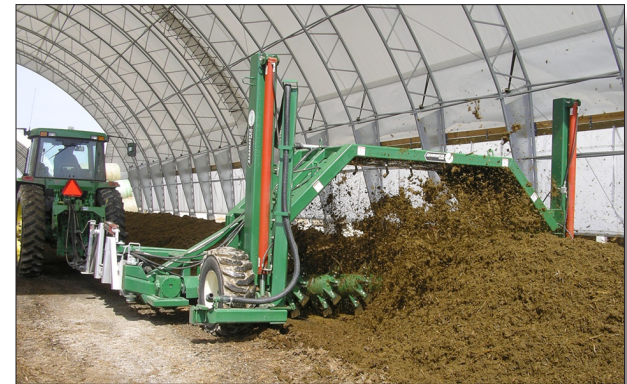
This machine turns and aerates a windrow.
